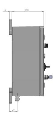
The four wall mount brackets can be placed horizontally or vertically, or using a horizontal/vertical combination.
