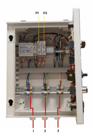
**1** • 2x2.5mm² or 2x1.5mm² cable. Connection of the 2 pilot wires (L' and L'') (right  $\frac{1}{2}$  stadium & left  $\frac{1}{2}$  stadium)
